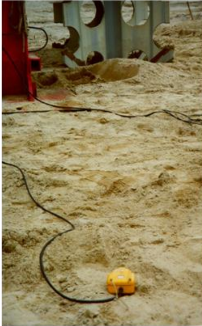
Fig. 10.13. Ground vibrations measured adjacent to the compaction probe,
