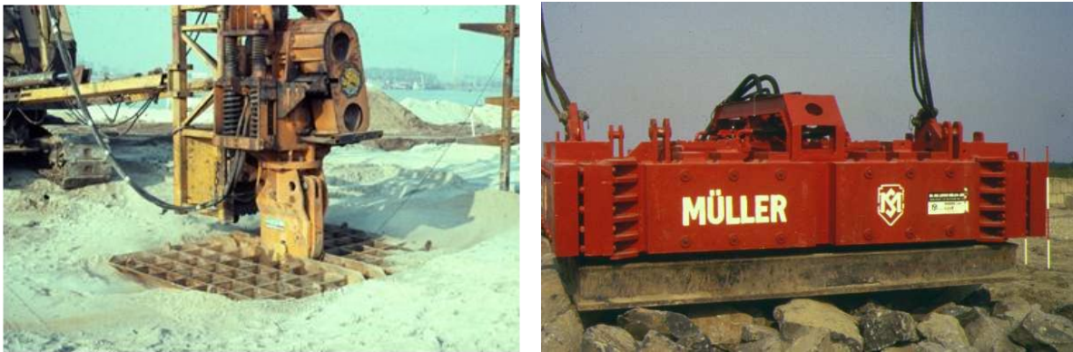
Fig. 10.6. Two types of vibratory compaction plate vibrators (operating at variable frequency).
