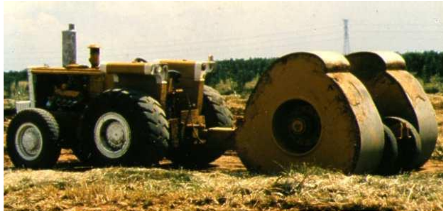
Fig. 10.5. Impact roller for deep compaction.
