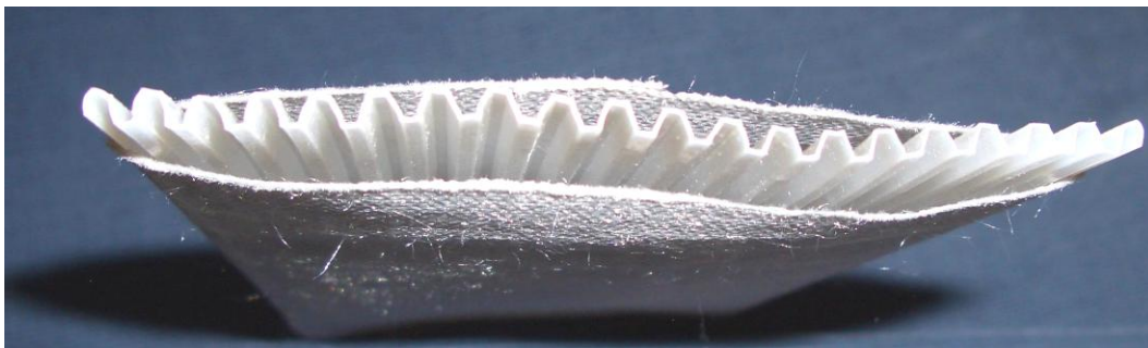
Fig. 5 Photo of the wick drain used for the project
